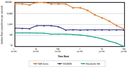
Figure 5. Update rates of popular oscilloscopes using their default real-time acquisition mode
